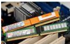
4GB DDR2 Wafer level package Memory Module -World Wide 1 st (2008.12)
